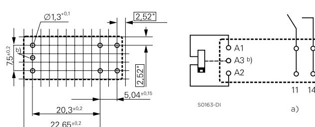
\*) With the recommended PCB hole sizes a grid pattern from 2.5mm to 2.54mm can be used.
