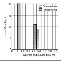
5-(1). Electrical life test (Resistive load) Sample: ACY11312, 6pcs. Load: Resistive load (NO side: 30A 14V DC Operating frequency: (ON: OFF = 1s: 9s) Ambient temperature: Room temperature
