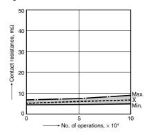
5-(2). Electrical life test (Lamp load)
