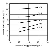
1-(2). Coil temperature rise (at 85°C 185°F) Sample: ACY11312, 3pcs Measured portion: Inside the coil Ambient temperature: 85°C 185°F
